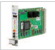
Modbus RTU gateway A serial interface card for connection to third party systems, including Dräger Vision32
