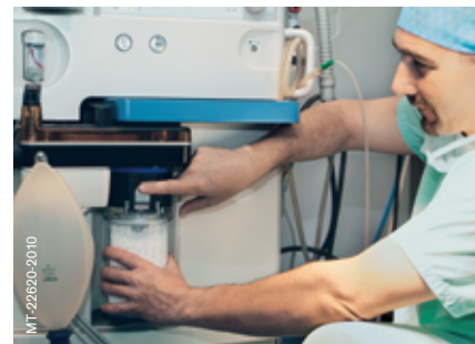
Replacing the absorber is easy and possible anytime, even during an operation.
