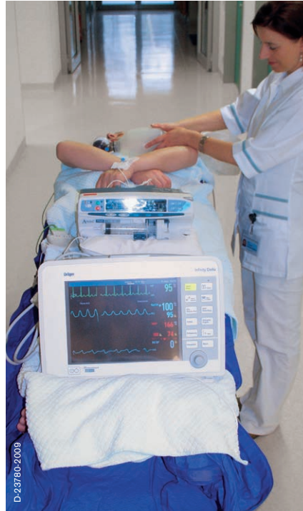
Fig. 6: Transport from induction room to radiation unit. The pick-and-go technology changes the Delta patient monitor into a transport monitor.
