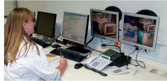
Fig. 7: Radiation control room. Two cameras in the treatment room deliver the images of the radiation directly to the control room for observation by the anesthetist.
