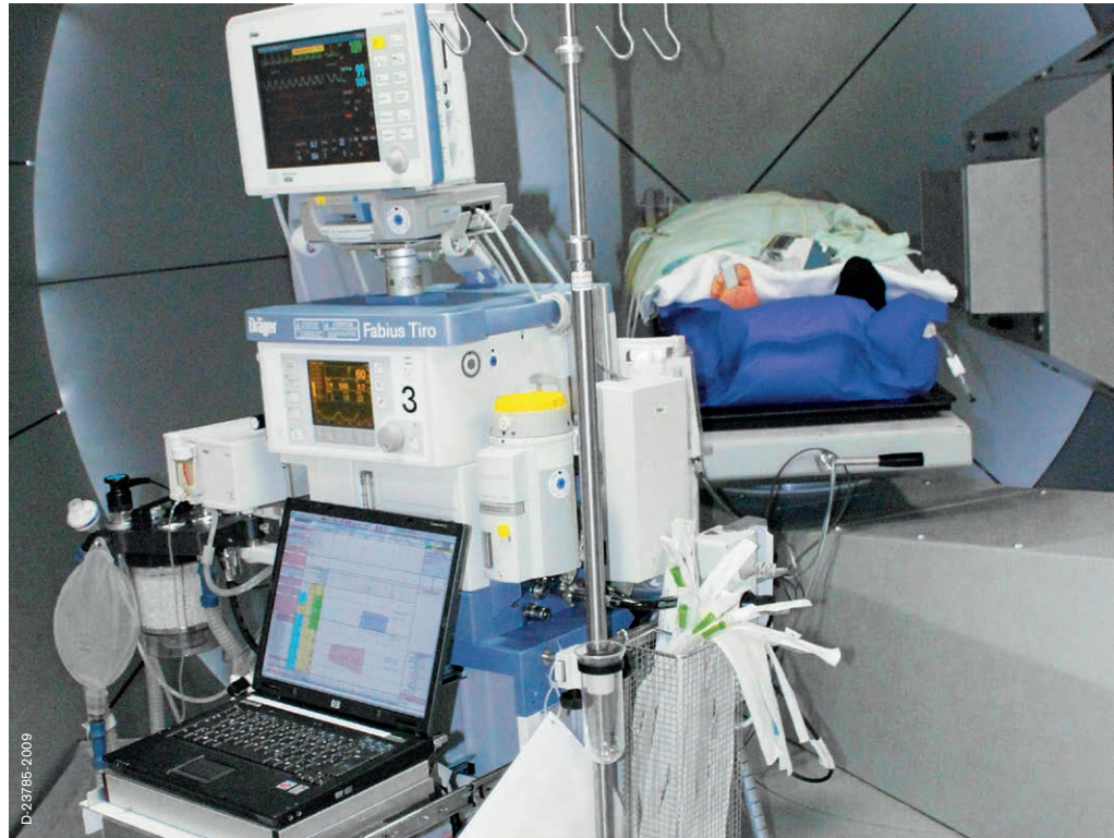
Fig. 11: Radiation room. The patient is connected via long breathing hoses in the radiation room to the Fabius Tiro anesthesia device. The doctors can determine with x-ray images via the flat panels on the nozzle whether the tumor is positioned precisely on target or not.
