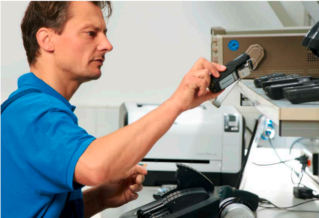
Much more convenient than manual exposure to gas: bump test at a test station.
