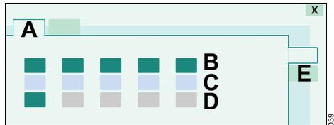
The set alarm limits and the current measured value are displayed.
