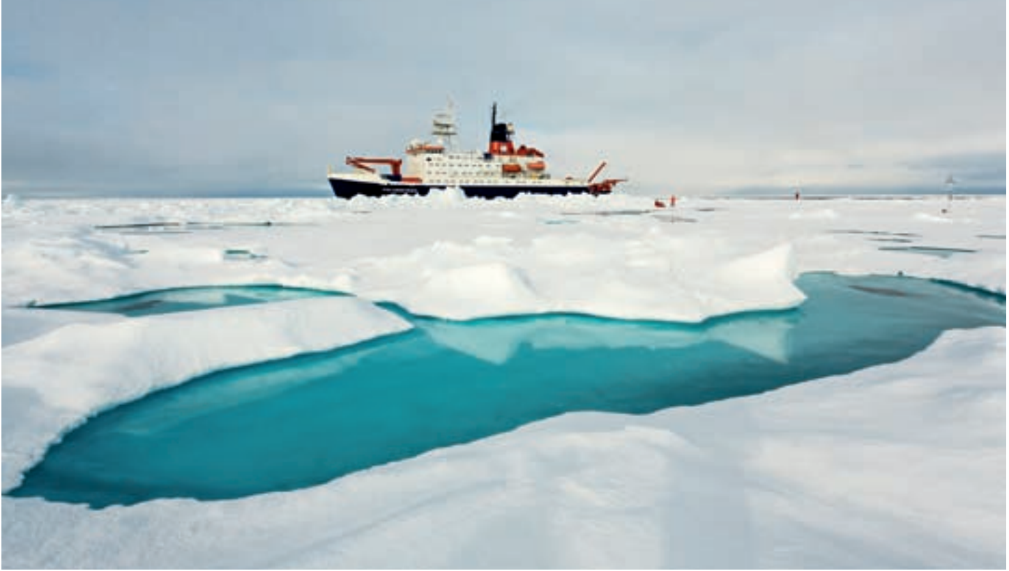
Home on the horizon: the Polarstern is 118 meters long and equipped with four engines with a total power output of 14,000 kilowatts (20,000 PS), and is one of the world's few research ships built as an ice-breaker
