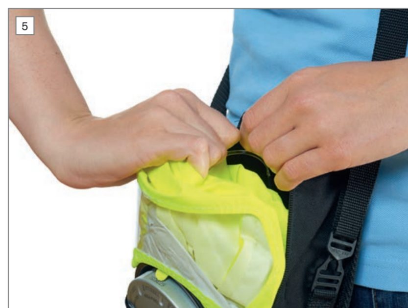
Remove the hood from the Soft Pack. Pull the hood against the fastening strap, it will automatically open. The second filter sealing plug will automatically be detached when the hood is removed.
