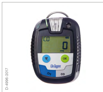
Dräger Pac® series 6000/6500/8000 and 8500 The new Dräger Pac 8500® single-gas detection device is a reliable and precise instrument even under the toughest of conditions. The device can be equipped with a hydrogen-compensated CO sensor or a Dräger dual sensor. This gives you the option of measuring two gases at once: either H2S with CO or O2 with CO.
