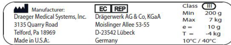
Fig. 5 Label with manufacturer information and scale accuracy class/weighing range information
