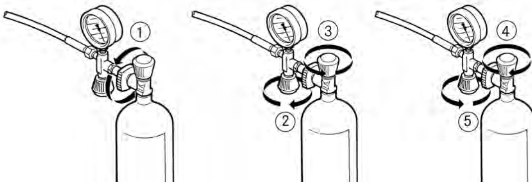
Fig. 19 Filling the compressed air cylinders
