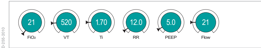
Figure 4: Possible ventilation settings for volume-controlled ventilation modes for adult patient category
