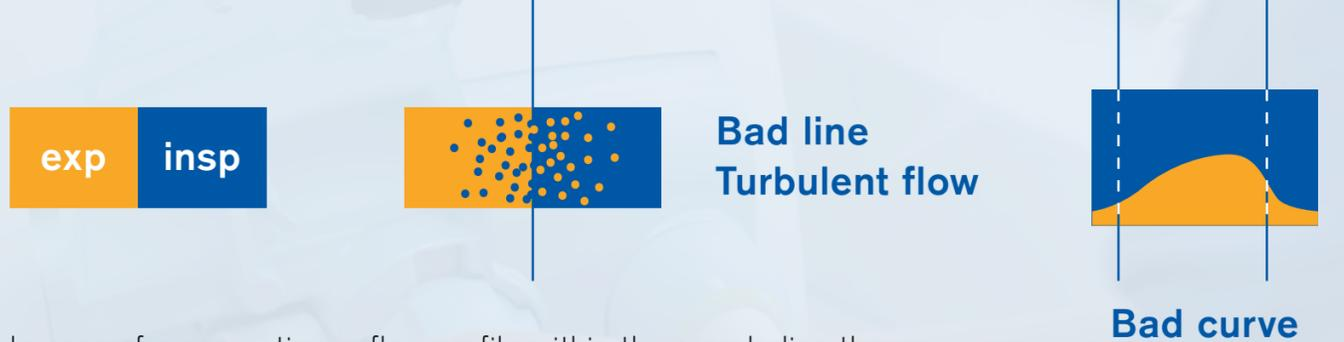
In case of a non-optimum flow profile within the sample line the real-time curve profile will be impaired. The "high" numerical values get false low, the "low" false high. **See image 2.**
