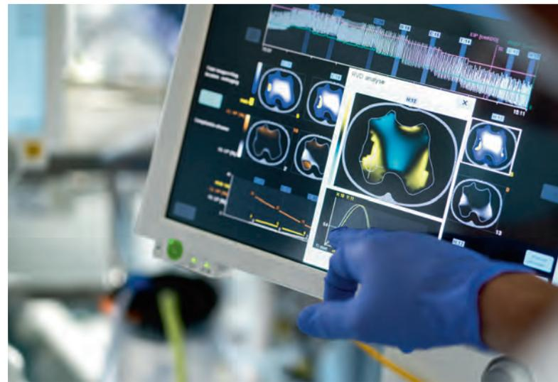
**BESIDES REAL-TIME VISUALIZATION**, the machine also works out the extent to which areas of the lungs are overdistended or collapsed
