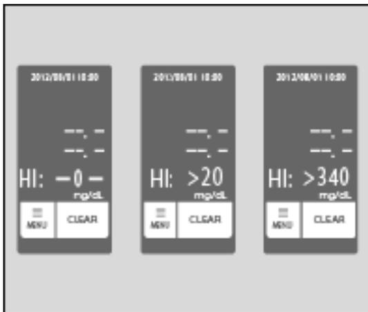
NOTE: To change this setting to blinking zero (HI: -0-), refer to the instructions for use. It must be changed using the data transmission software, SW JM-S1w. Requires JM-S1w version 1.40 or higher.
