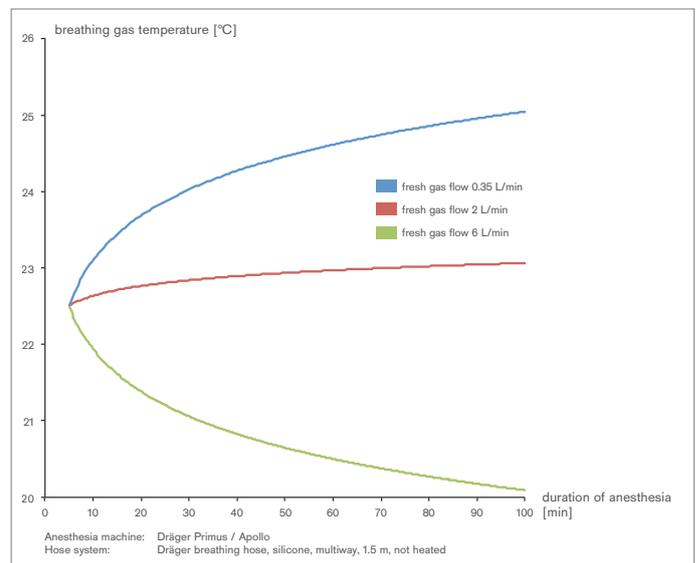
Breathing gas temperature in °C measured at the Y-piece in the inspiratory arm of the Dräger Primus / Apollo anesthesia machine over the course of anesthesia
