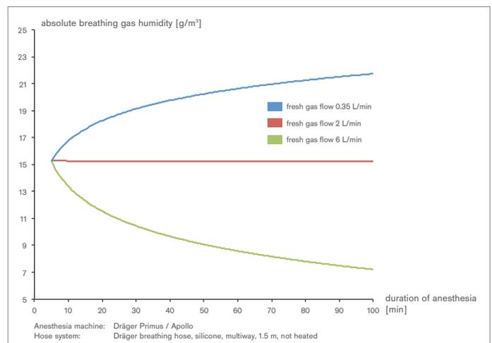
Absolute humidity in g/m<sup>3</sup> measured at the Y-piece in the inspiratory arm of the Dräger Primus / Apollo anesthesia machine over the course of anesthesia
