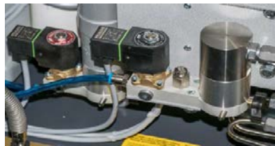
Automatic condensate drain system
