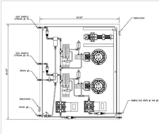
If the pressure were too high or too low, a **pressure regulator** would be added to the system to bring the sample pressure to near ambient before it reaches the system. In cases where the gas may over range the sensor on occasion, a dilution system can mitigate the problem by lowering the gas level to acceptable levels. Over-ranged sensors can have long recovery times that cause inaccurate measurements for a period of time, or may stress the sensor so a calibration is required.
