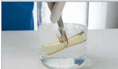
Immerse flow sensor bubble-free in the cleaning solution for the agent specific exposure time.
