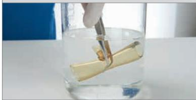
Repeatedly swirl the flow sensor in the disinfection solution for the agent specific exposure time. Ensure that the solution flushes all surfaces and interior spaces.
