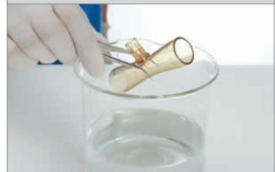
Allow the flow sensor to air dry for at least 30 minutes.
