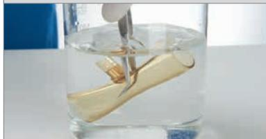
Ensure that the cleaning solution flushes all surfaces and interior spaces.
