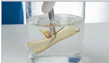
Inspect flow sensor for visible soiling and damage.
