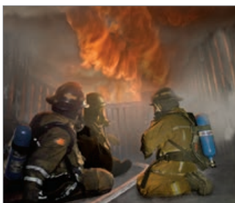
Thermal layering, as observed in the chamber.
