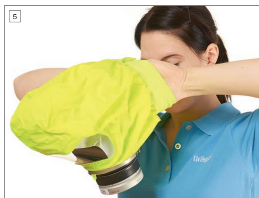
Widen the neck seal and pull the hood over your head. The inner head harness automatically adjusts to your head. Ensure that nose and chin sit comfortably in the half mask and that all hair is tucked into the hood.
