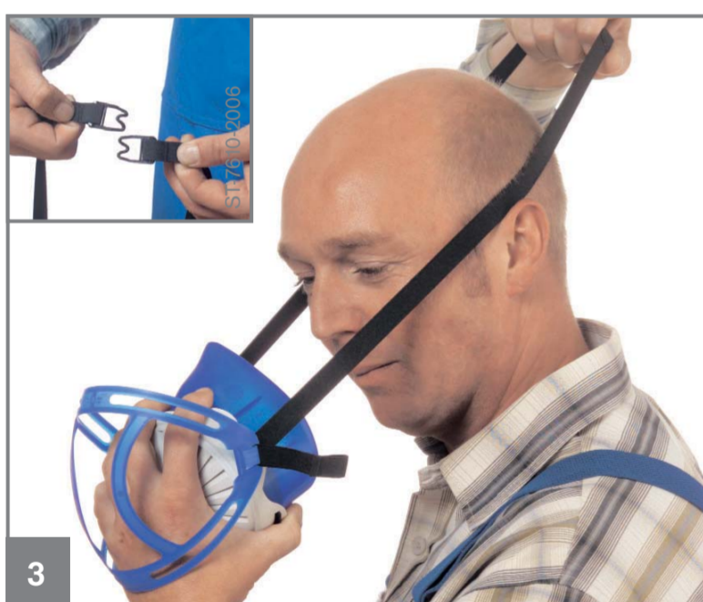
3 Connect the hooks on the neck strap and place the straps at the back of the neck.
