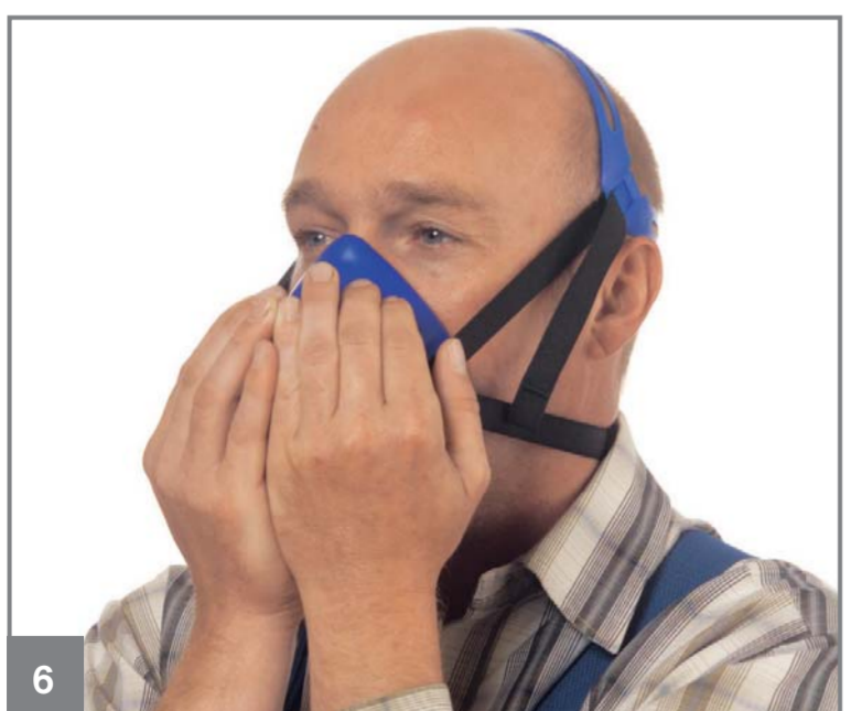
6 Seal respiratory filter cap with your hands and exhale. The half mask will inflate slightly. If the exhaled air leaks out of the mask, readjust the face-piece and adjust the straps or use a different size. Repeat test until a successful seal check is met.
