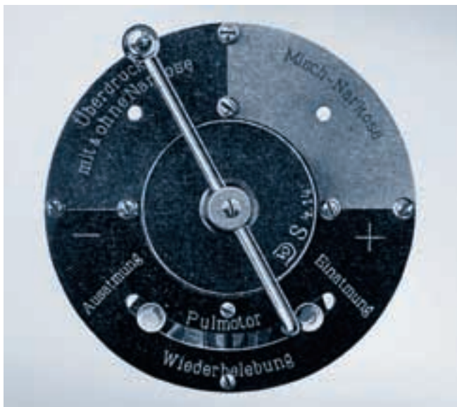
The selector or switching valve on the same apparatus.
