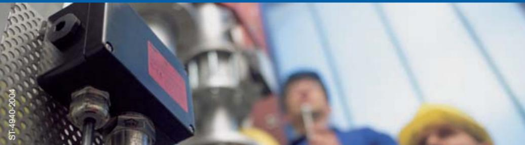
Under certain circumstances flammable gases and vapours can be oxidized by means of the air's oxygen to release heat of reaction. Typically this is achieved by special and suitable heated catalyst material, which slightly increases its temperature by the heat of reaction. This increase of temperature is a measure for the gas concentration.
